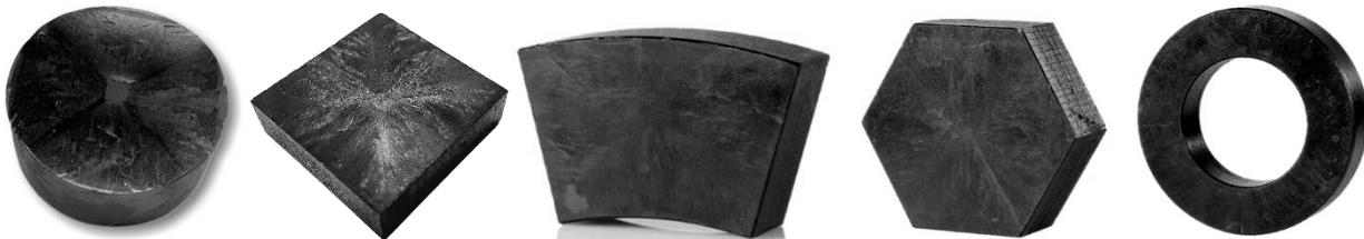
**Material:** Melt textured REBa<sub>2</sub>Cu<sub>3</sub>O<sub>7-x</sub> with RE<sub>2</sub>BaCuO<sub>5</sub> excess
